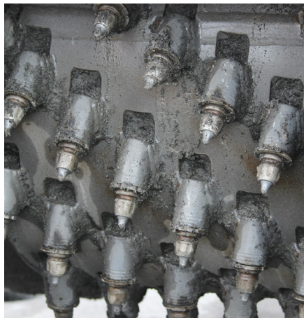
Head of the milling machine after milling.
