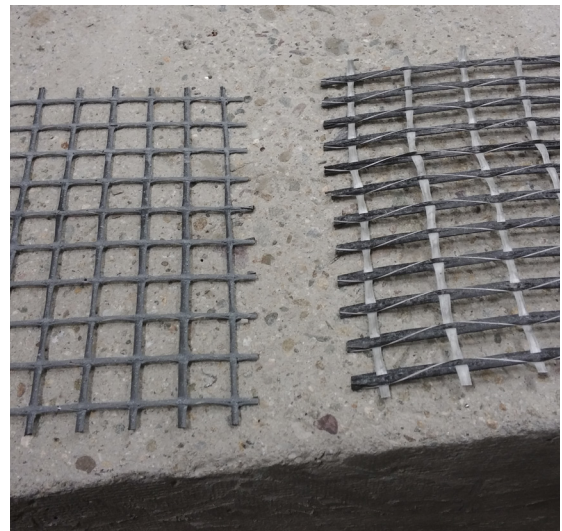
Bidirectional (left) and unidirectional grid (right).
